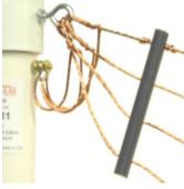
Cut each of the wires leaving about 4 inches long pigtail. Then attach the terminals to each wire. Put 2 terminals on the stud. Tighten one nut. Put the remaining 2 terminals on the stud, tighten another nut. Repeat for the other side of the dipole.
